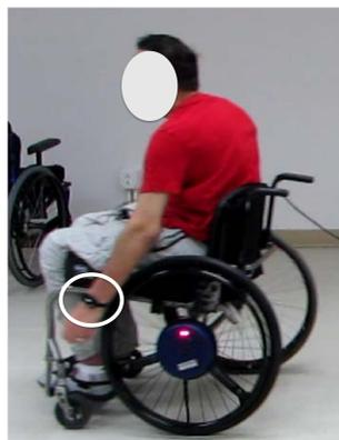
**Figure 4:** Propulsion data collected from wrist-worn sensor and instrumented pushrim from C7 AIS B SCI MWC user
